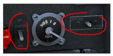
clutch which connects flywheel to the engine's crankshaft.
