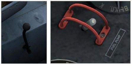
provide a back-up for the engine-driven fuel pump during take-off and landing.
